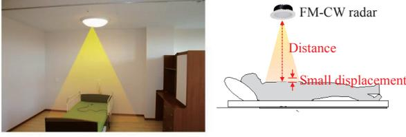
**Figure 8: An setting example of FM-CW Radar for detecting human breathing**
