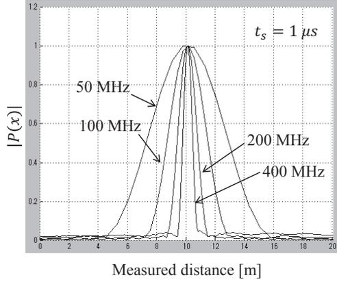
Fig. 3. Resolution for distance spectrum according to sweep bandwidth.
