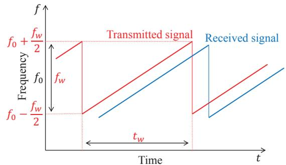
Fig. 1. Sawtooth frequency modulation.
