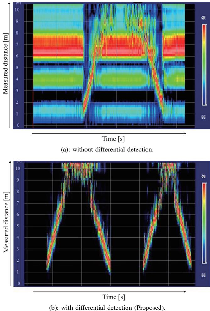
Fig. 8. Distance spectrum for measuring moving target distance with / without the differential detection.
