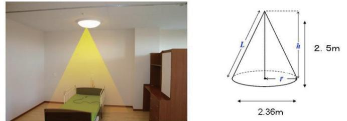
Fig. 10. Setup of FM-CW Radar for detecting human breathing.
