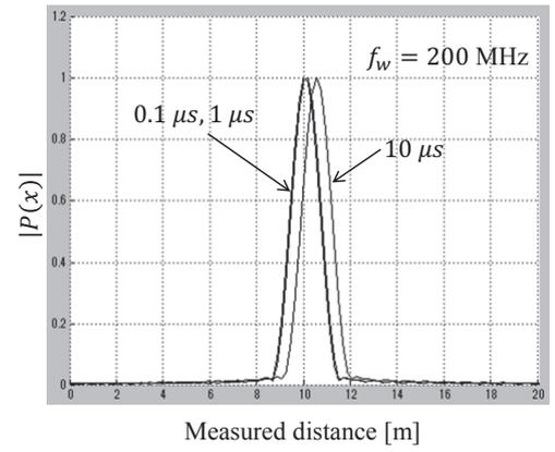
Fig. 4. Error value for distance spectrum according to sampling interval.
