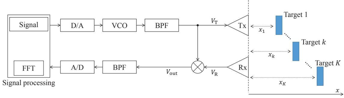
Fig. 2. Block diagram of a FM-CW radar system.
